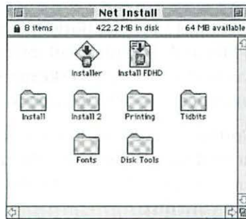
Figure 2.5 A locked disk has a padlock on the top left of the disk window.
