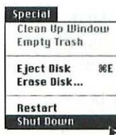
Figure 2.2 To turn off the Mac, choose Shut Down under the Special menu in the Finder.
