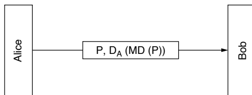
Figure 8-23. Digital signatures using message digests.
